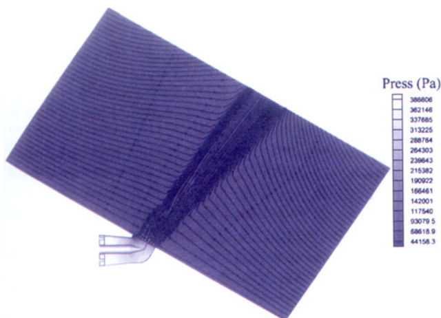
Fig. 8 Streamline patterns in the plane of symmetry of the aircap and exterior
