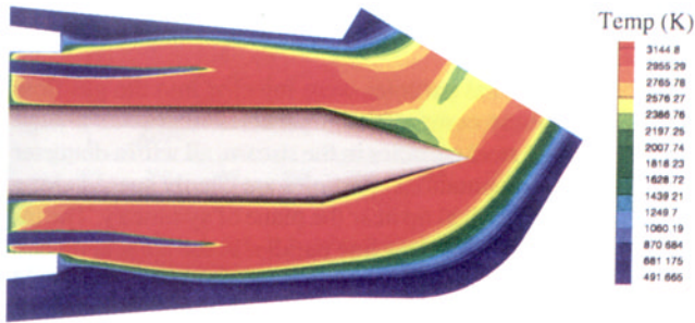
Fig. 4 Plane of symmetry gas temperature contours inside aircap
